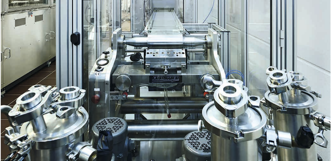
Technology development for multilayer coating using triple-slot-die coating.
