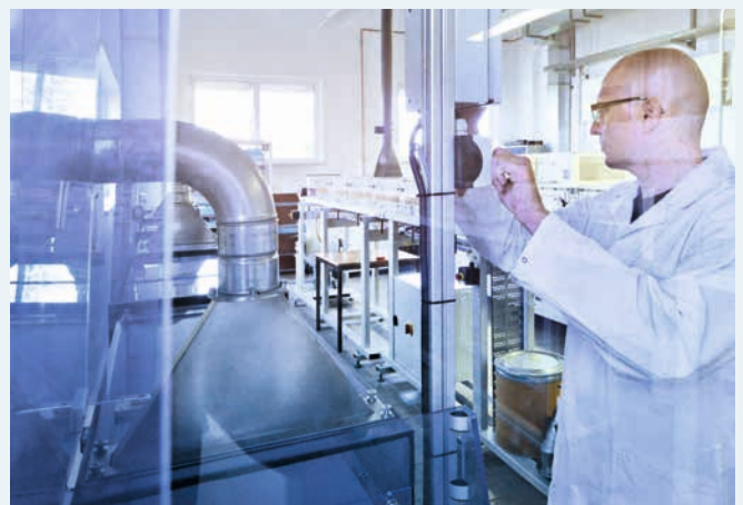
Slot-die coater in the tape casting center at the Hermsdorf site.
