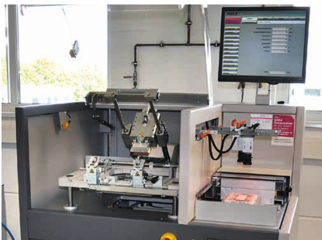
EKRA-M2H screen printing machine for functionalization of ceramic tapes.
